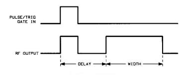
This modulation source requires an external trigger source.
